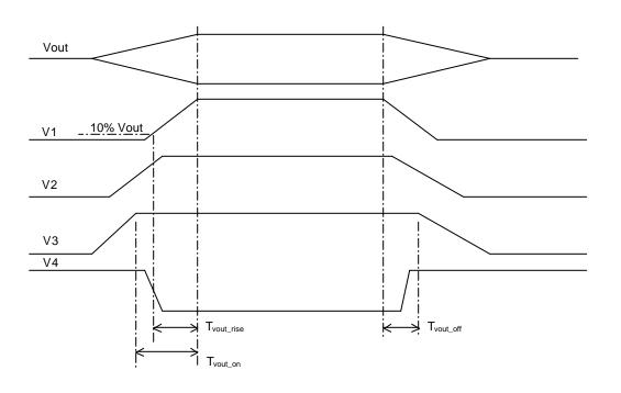
Figure 2: Output Voltage Timing
